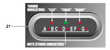
**21. ELECTRONIC TUNER (top panel):** The electronic tuner is active whenever the amplifier is turned on, providing constant, "real-time" tuning. The bottom row of LEDs indicate which note (string) is being tuned. The top row of LEDs provides directional queues to facilitate quick and precise tuning of your instrument. The indicated note (string) is properly tuned when only the center LED is illuminated.
